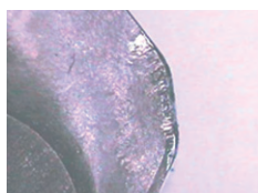
ZCC·CT insert after 80 minutes machining
