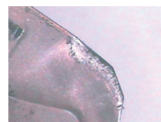
Insert of company A after 48 minutes machining
