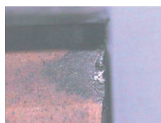
Insert of company A after 48 minutes machining
